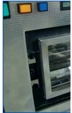
Figure 2: SteriBeam desktop intense pulsed UV system for 360° illumination of samples
