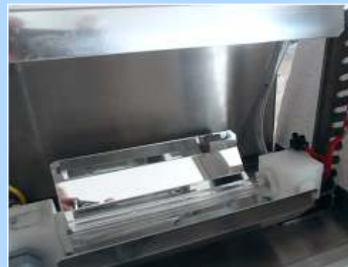
Two horizontal water cooled PUV modules and UVC transparent shelf between.
